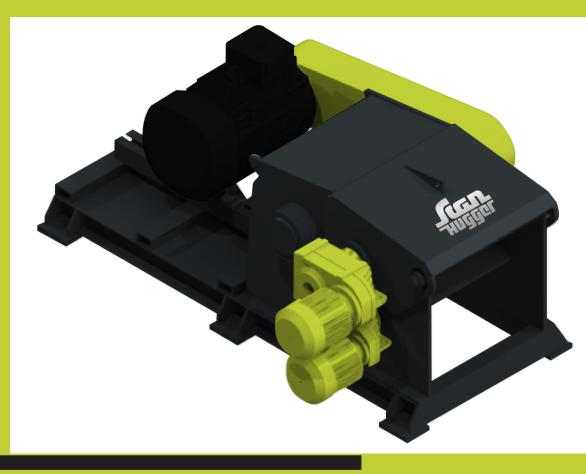
The horizontal shredder is available with two cutting systems. The standard rotor system is a solid, precision machined steel drum ideal for chipping solid wood slabs, edgings, and off-cuts to a defined chip size. The second rotor system is a solid steel drum with a precision mounting arrangement of four-sided knife blocks ideal for processing particleboard, MDF and plywood scrap.
